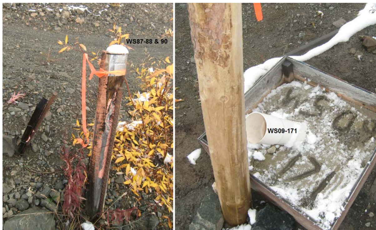
Figure 12.1: Drill Hole Collar Markers
